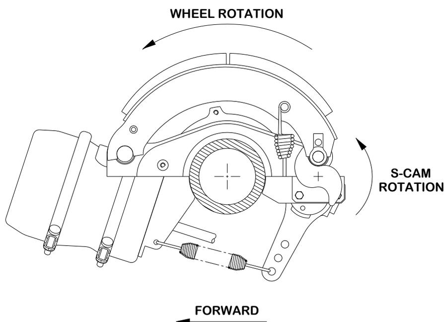
Failure to comply with this recommendation by having the S-Cam rotating against the direction of the wheels when travelling forward (reversed S-Cams) may result in noisy brakes, premature wear of the brake linings and premature wear of the tyres.
