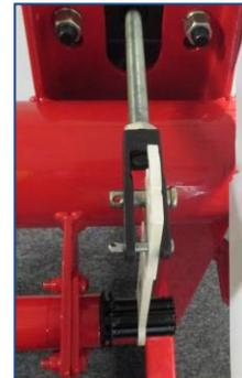
2. Screw the clevis in or out until the ¼" clevis pin can be installed without force (with the ½" pin still installed).
