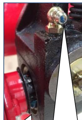
Keep pumping grease until it purges out on to the spline.
