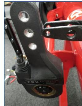
8. With 7/16” socket or ring spanner (**do NOT use an impact gun**) rotate the manual adjuster clockwise until the clevis holes line up with the holes on the ASA. Insert the ½” and the ¼” clevis pins (without using any force) and secure them with the split pins.
