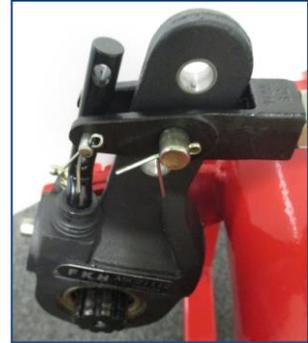
7. Install the washers and snap ring and allow the ASC a minimum of approx. 0.5mm to 2.0mm lateral movement on the spline.
