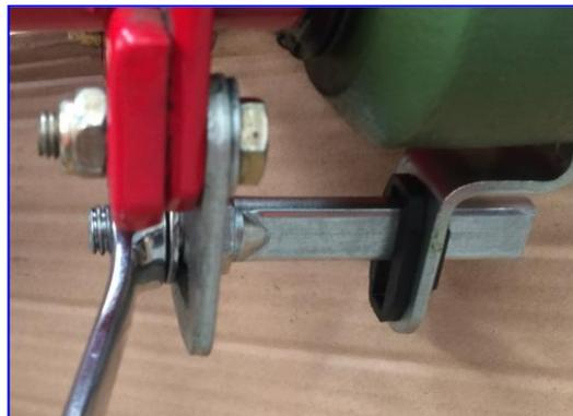
7. With the 12mm socket (spanner), rotate the manual adjuster clockwise until the brake shoes contact the brake drum.
