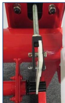
2. Screw the clevis in or out until the ¼" clevis pin holes line up (with the ½" pin still installed).
