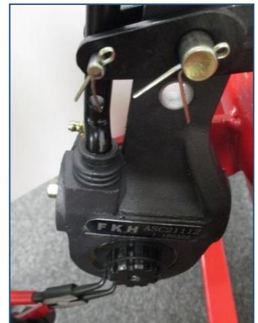
8. For the final adjustment turn the manual adjuster with the 7/16" socket clockwise until all the slack is been taken up (without excessive force) and then do a 1/2 turn anticlockwise.
