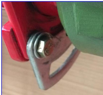
2. Clean the s-cam spline and apply some lube on to the spline before installing the ASH.
