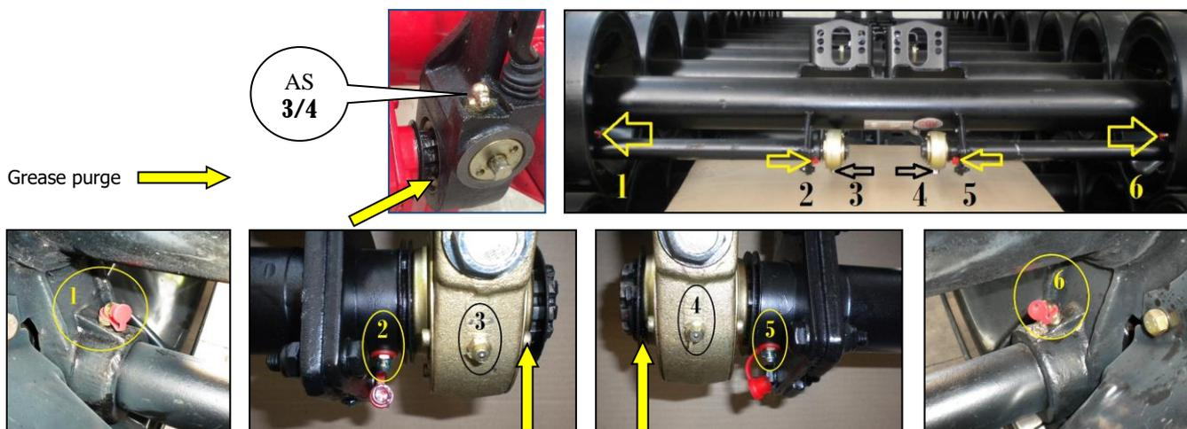
**Note:** When greasing the 6 grease nipples the very 1<sup>st</sup> time it is important to **fill** the grease channels and cavities.
