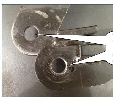
The hole in the top and bottom levers must be Ø16mm.
