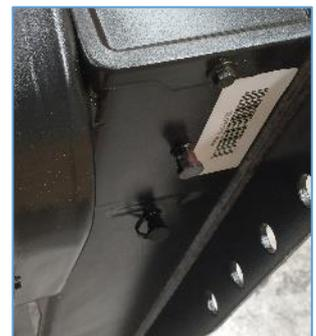
5. Periodically (annually) remove the plastic cover and check (replace) the grease in the gearbox.
