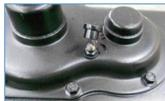
5. Periodically (annually) remove the plastic cover and check (replace) the grease in the gearbox.
