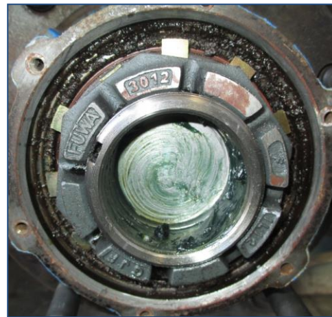
This seal is leaking – Replace the Bearing!
