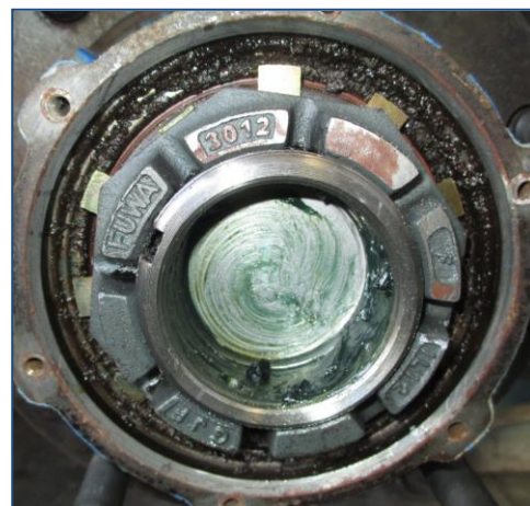
...a large amount of grease is visible...
