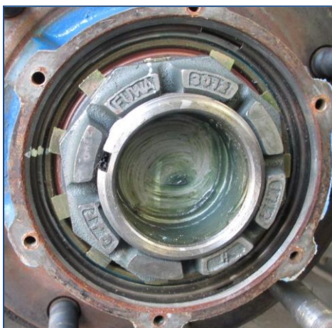
...no grease is visible...
