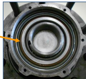
The O-Ring is on the bearings inboard side.
