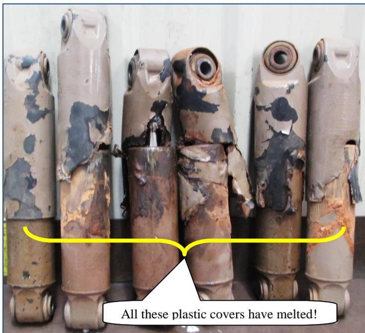
The plastic covers on these particular shock absorbers will start to melt after being exposed over 1 hour at approx. 200° C.
