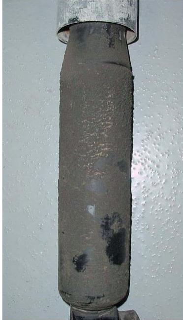
Heavy oil/dirt film extending to the bottom of the damper
