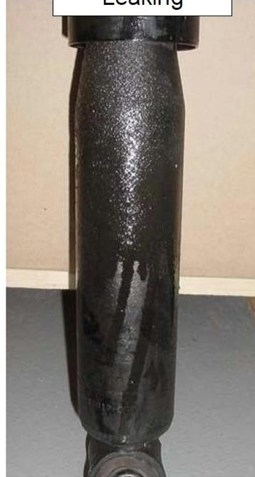
Oil leak path lines visible on damper
