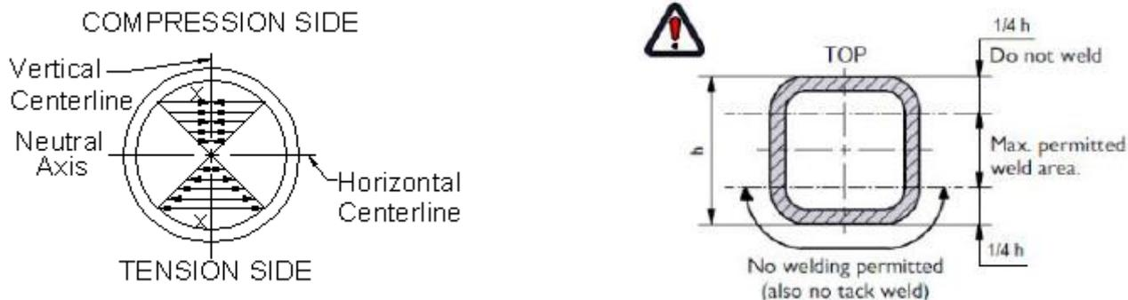
Figure 1 Degree of stresses on the axle beam
