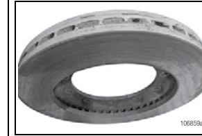
Clogged Vent Holes FIGURE 116
