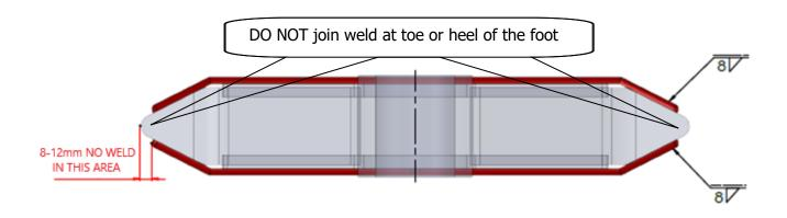
**Base plates** should be attached to the vehicle strictly in accordance with the (AS/VSB) standards as per table below: Nuts and bolts shall be M16 (5/8") or M20 (3/4"), Class 8.8 (SAE Grade 5) minimum.
