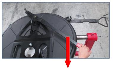
3. Unhook the pivot, and lift the tool off the 5<sup>th</sup> wheel.
