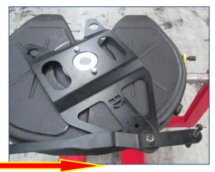
....by moving the tool from side to side, you can feel the tightness of the jaw on the king pin.
