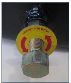
"ADJUST FOR WEAR" means the king pin is loose.
