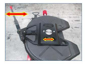
Unhook the lever pivot point from the front of the 5<sup>th</sup> wheel .....
