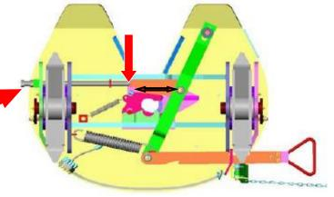
NOTE: Only the single jaw  $5^{\rm th}$  wheel (KA & KC) can be adjusted. The two piece jaw  $5^{\rm th}$  wheels (KH) cannot be adjusted.
