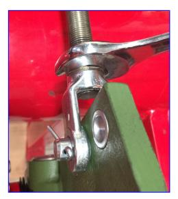
4. Install the outer washer and snap ring and allow the ASH a minimum of approx. 0.5mm to 2.0mm lateral movement on the spline.
