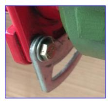
2. Clean the s-cam spline and apply some lube on to the spline before installing the inner washer then the ASH.
