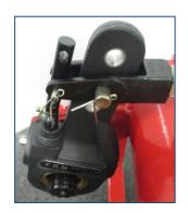
7. Install the outer washer and snap ring allowing the ASC a minimum of approx. 0.5mm to 2.0mm lateral movement on the spline.
