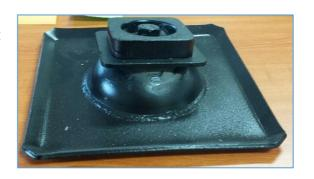
a. Grind off the weld connection of the old foot to the main landing leg body.
