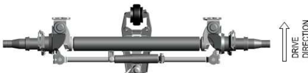
fig. No.16 Self-steering axle with 1 shock absorber (top view)
