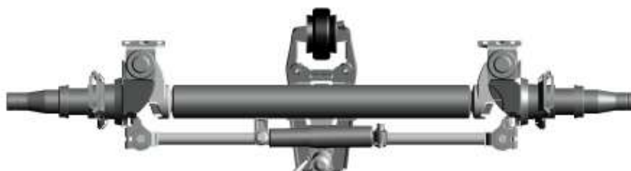
fig. No.10 Rear rod self-steering axle (top view)
