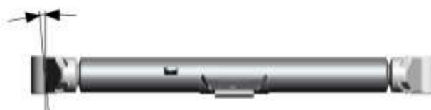
fig. No.23 (rear view) positive camber
