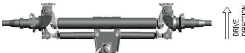
fig. No.17 Self-steering axle with 2 shock absorbers without stabilizer (top view)
