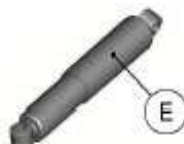
Fig. No. 15 Shock absorber
