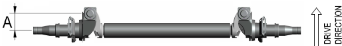
fig. No.2 Self-steering axle (top view)
