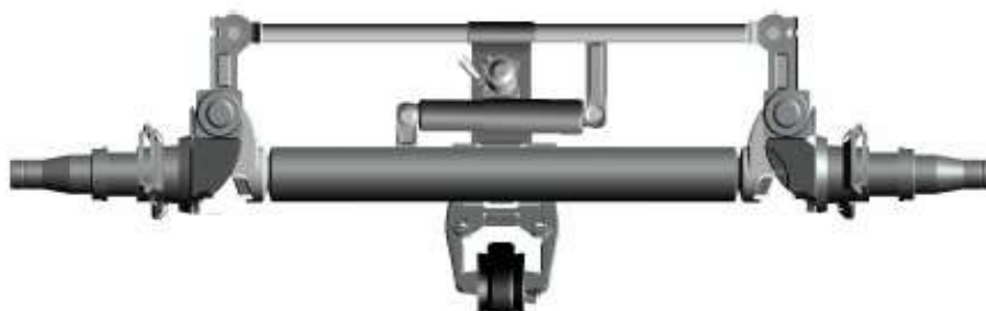
fig. No.11 Front rod self-steering axle (top view)
