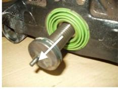
Remove dust cap from the caliper tight fit with a screw driver.
