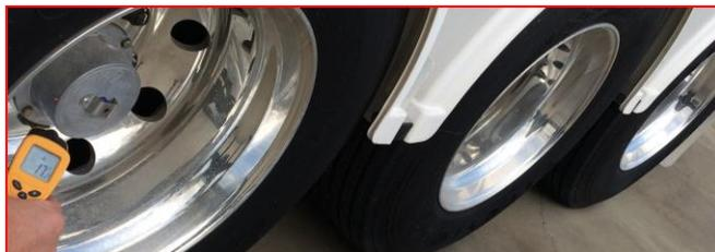
Rather than touching the hub by hand, we strongly recommend the use of an electronic infrared thermometer.
