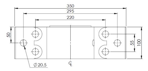
The feet can only be bolted to the base plate with: **M20x1.5 10.9** bolts torqued to 600Nm (dry).
