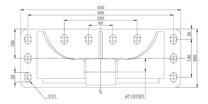
The feet can be bolted to the base plate with: M20x1.5 10.9 bolts torqued to 600Nm (dry).
