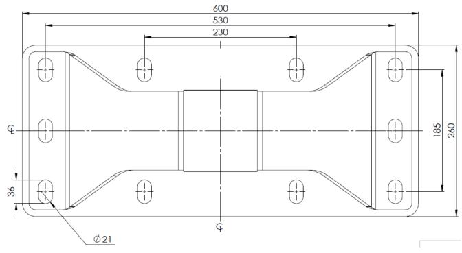
The feet can be bolted to the base plate with: M20x1.5 10.9 bolts torqued to 600Nm (dry).
