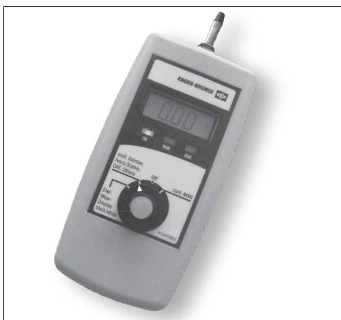
5.1.13 - Knorr-Bremse diagnostic unit K154433N50
